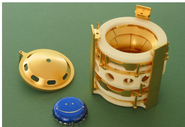
Fig. 2. The LEBIT high-precision Penning trap with the endcap electrode removed. Note the eight-fold segmentation of the hyperbolic ring electrode.
